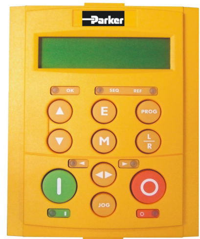
SEQ and REF LEDs are On when in Local mode
