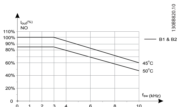
Illustration 5.11 Output Current Derating with Switching Frequency and Ambient Temperature for 600 V Frequency Converters, Enclosure Sizes B, 60 AVM, NO
