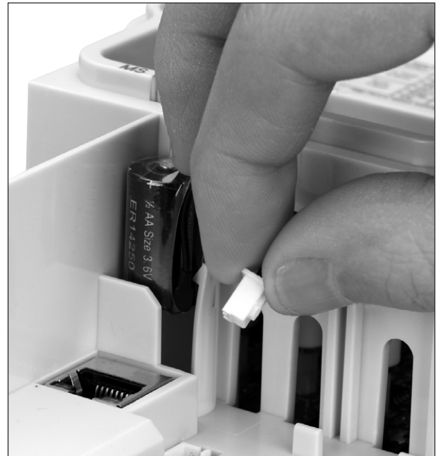
Figure 1. RTC battery connection
