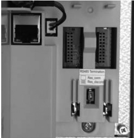
Figure 33. RS-485 Bus termination setup
