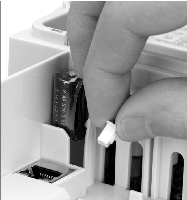
Figure 1. RTC battery connection
