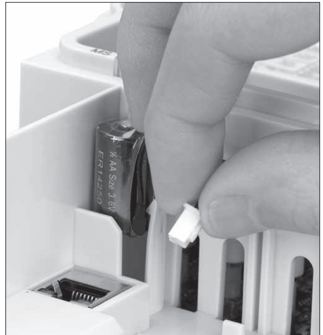
Figure 1. RTC Battery connection
