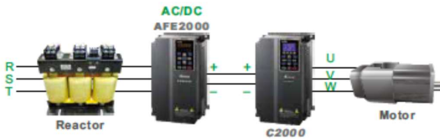
AFE with one Frequency drive
