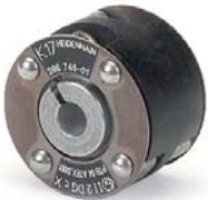
Diaphragm coupling K 17 with galvanic isolation For ROC/ROQ/ROD 400 and RIC/RIQ 400 series With 6 or 10 mm shaft diameter ID 296746-xx
