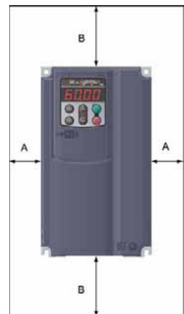
Figure 2.1 Mounting Direction and Required Clearances
