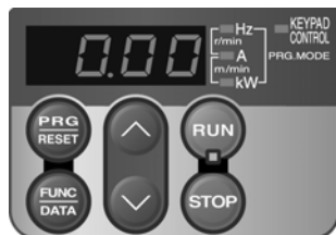
Figure 4.2 Display of the LED Monitor after Power-on
