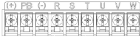
Figure 3-6: 3PH main circuit terminals (200V, \leq 1.5\text{kW} , and 380V, 4-22kW)
