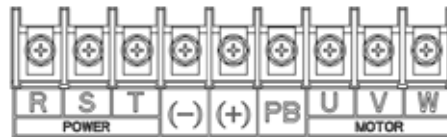
Figure 3-8: 3PH main circuit terminals (45-110kW)
