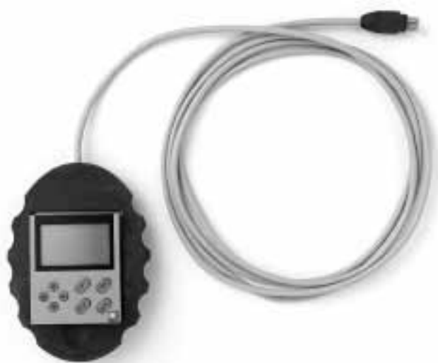
Hand terminal (handheld keypad and connecting cable)
