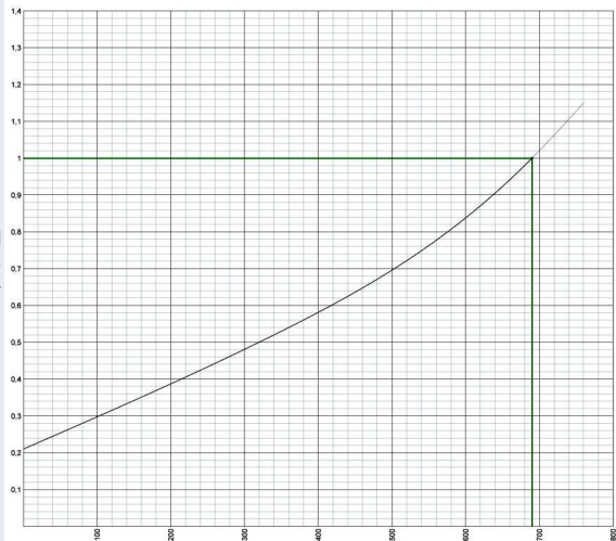
I 2 t multiplier coefficient 5 to 32A
