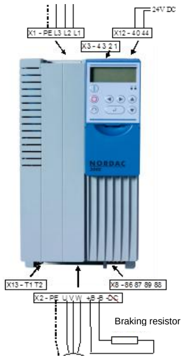
Figure 10: Power connection SK 5xxE up to size 7
