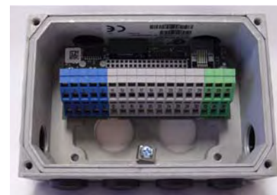
External BUS connection unit = SK TI4-TU-BUS
