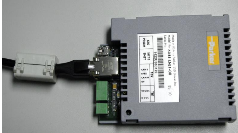
6055-LNET-00 TECHBOX with FERRITE CORE Installed
