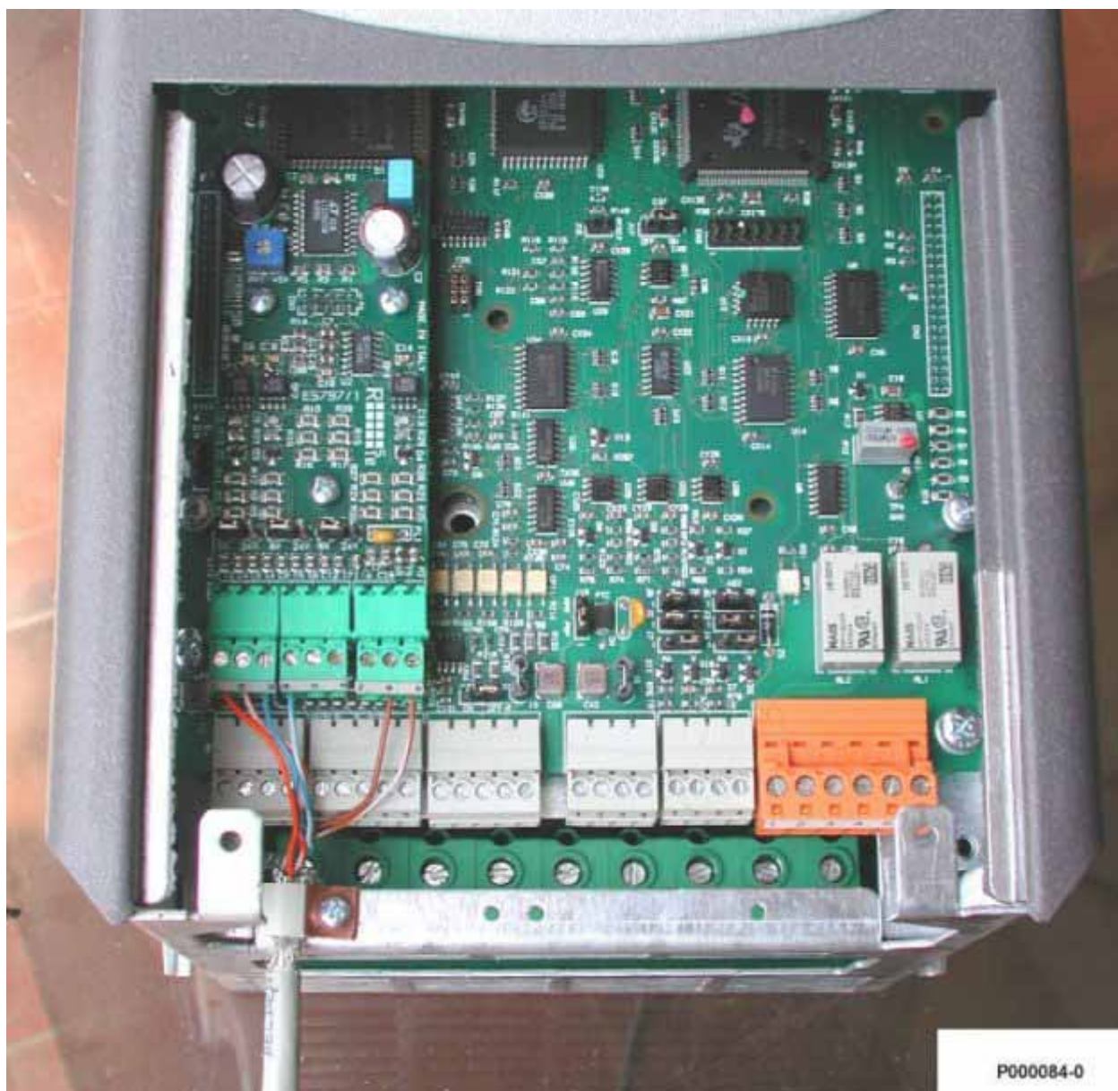
Figure 85: Wiring the encoder cable.
