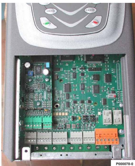
Figure 79: Encoder board fastened to its slot.
