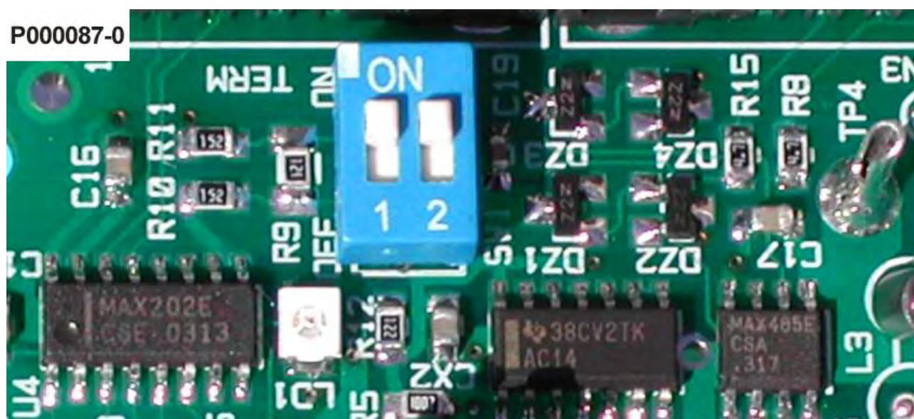
Figure 130: Configuration of terminator DIP-switch for line RS485
