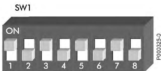
Figure 188: DIP-switch SW1 setting in three-channel mode
