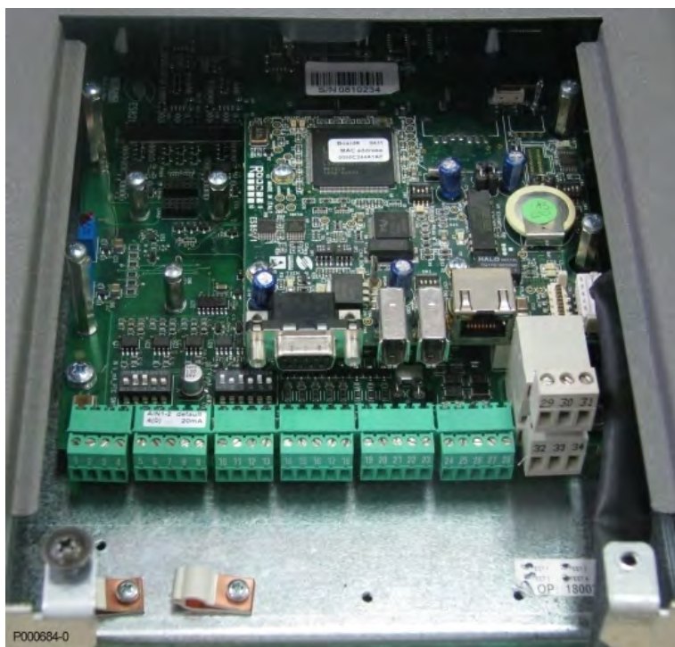
Figure 159: ES851 DataLogger fitted into slot B
