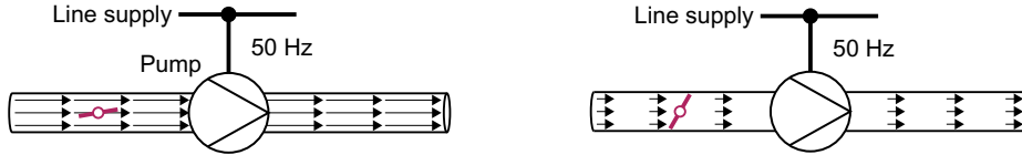
Figure 6-67 Flow control with pump and throttle connected to a 50 Hz line supply
