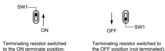
Figure 4-9 Switch Positions for Bus Terminating Resistors
