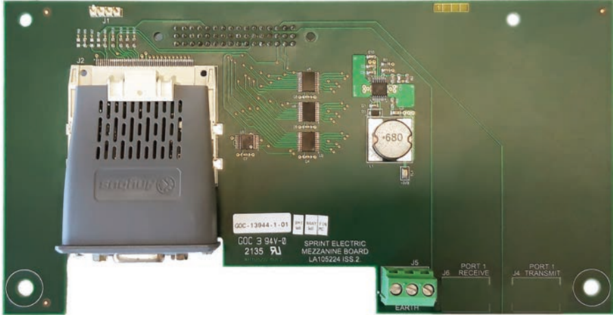
Figure 1 Fieldbus mounting board fitted with Anybus CompactCom module
