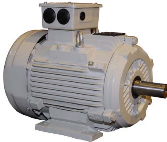
Figure 3-5: Multi- mount design (in axial direction); terminal box "Non drive end"
