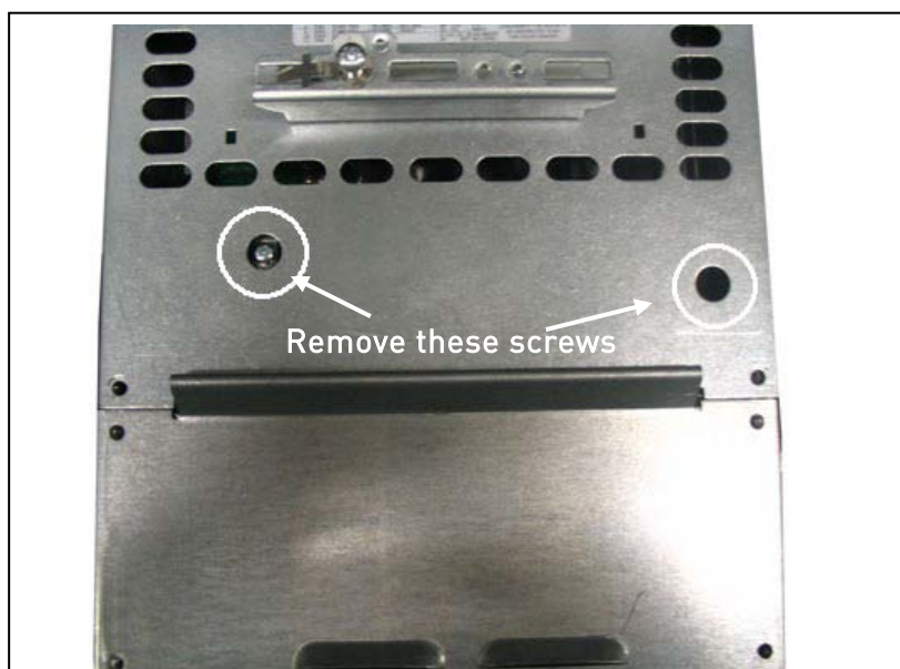
Figure 6-2. Changing of EMC protection class, FR4 (left) and FR5 (right). First remove the cable cover.
