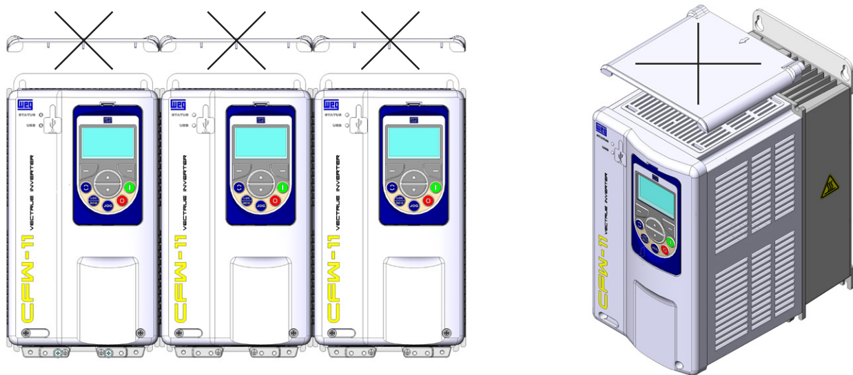
Figure 3.3 - (a) and (b) - Minimum side clearance requirements for inverter ventilation
