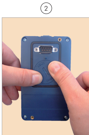
Press the cover and rotate it counterclockwise
