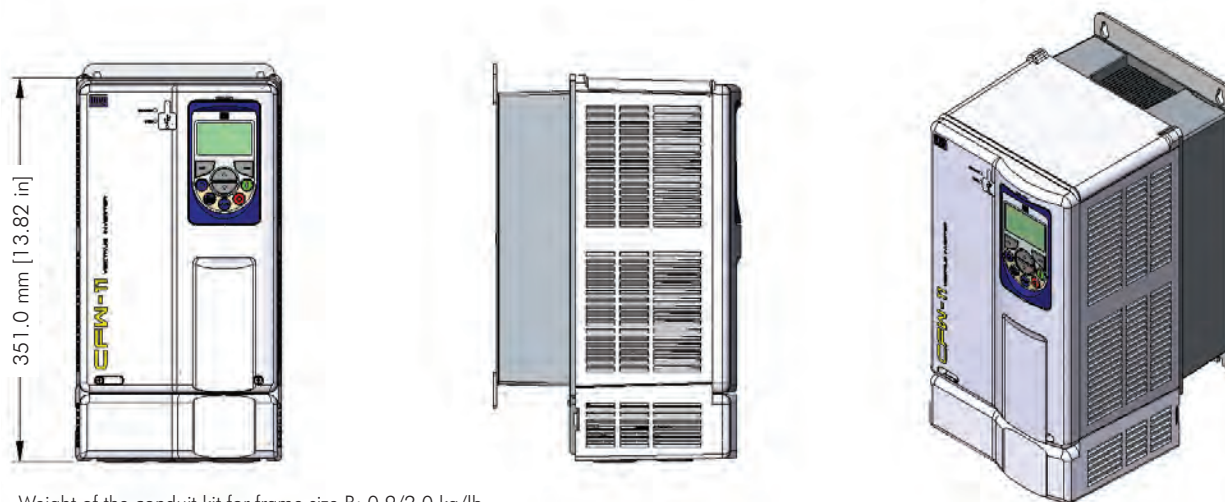
Figure 8.9 - Frame size B with Nema 1 kit KN1B-01
