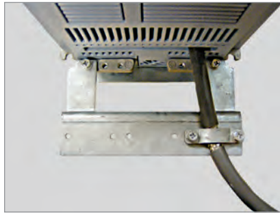
Figure 3.34 - Detail of the motor cable shield connection with the power cables shielding kit (PCSx-01) provided with inverters of frame sizes B and C
