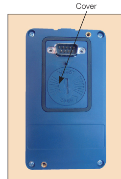
Figure 31: Keypad battery cover to access battery
