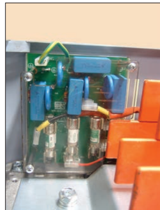
(b) Procedure for disconnecting the RFI filter and the MOV connected to the ground – necessary for using the inverter in IT or corner-grounded delta networks
