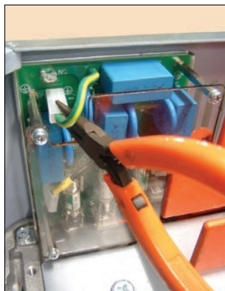
(b) Procedure for disconnecting the RFI filter and the MOV connected to the ground – necessary for using the inverter in IT or corner-grounded delta networks
