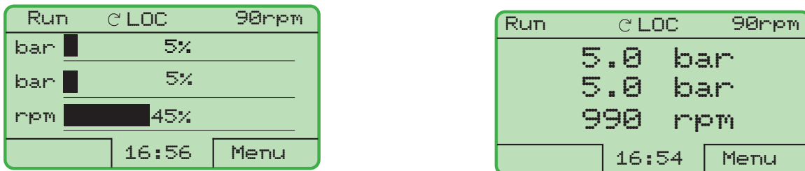
Figure 22.4 - Example of the keypad (HMI) in the monitoring mode for the PID Regulator function
