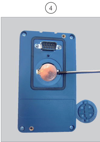
Remove the battery with the help of a screwdriver positioned in the right side
