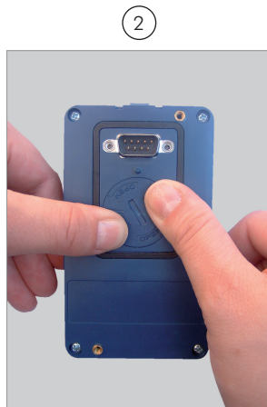
Press the cover and rotate it counterclockwise
