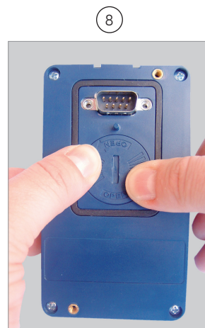
Put the cover back and rotate it clockwise
