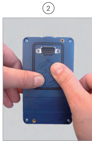
Press the cover and rotate it counterclockwise
