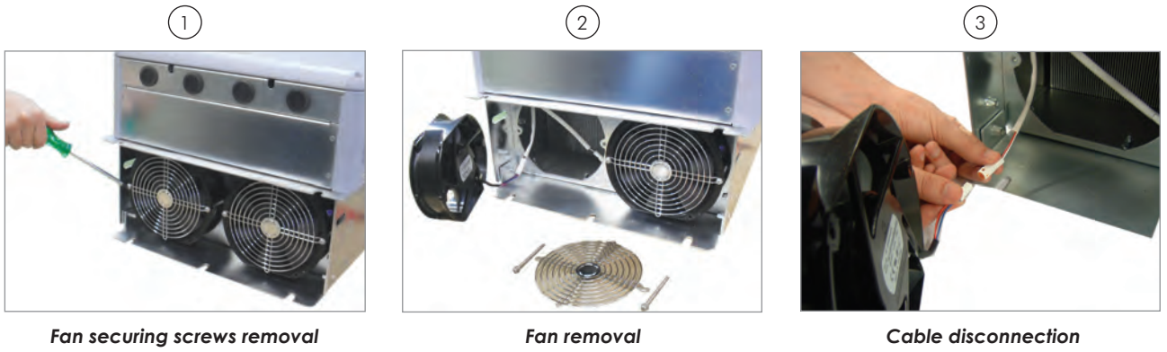
Figure 6.1 - Removal of the heatsink fans
