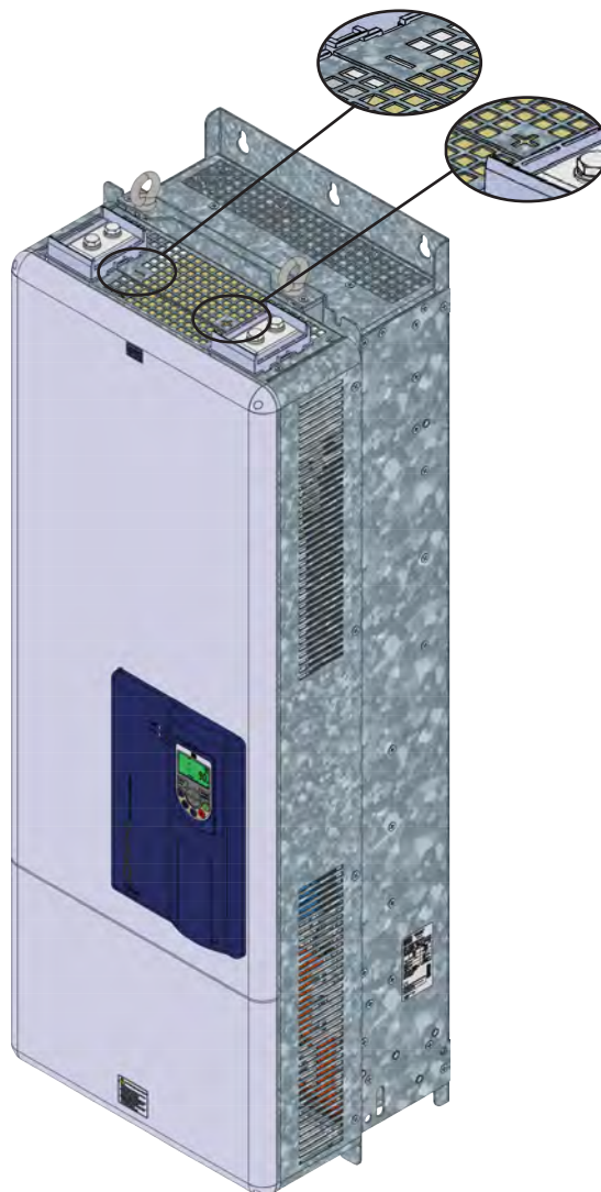
(b) Frame size F DC connection terminals (In models with special DC hardware, the R/L1, S/L2 and T/L3 terminals are not internally connected in this version)
