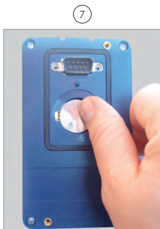
Press the battery for its insertion
