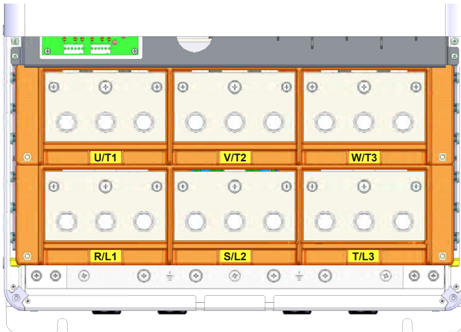
(c) Frame size G power terminals and grounding points
