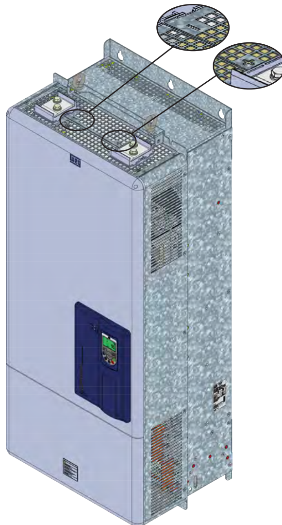
(d) Frame size G DC connection terminals (In models with special DC hardware, the R/L1, S/L2 and T/L3 terminals are not internally connected in this version)
