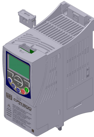
a) Removal of the STO jumper connector
