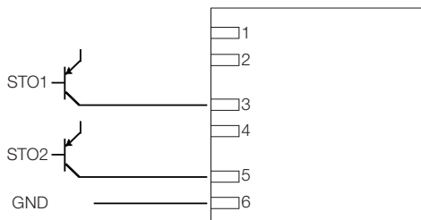
Figure 2.3: Installation using OSSD signals
