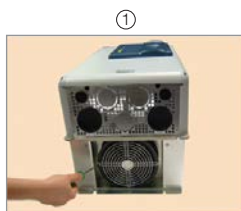
Removal of the fan grid screws
