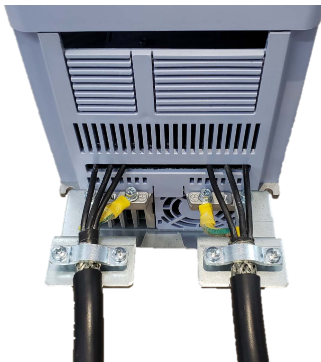
Figure 3.16: Detail of the motor cable shield connection
