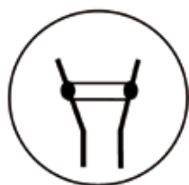
IEC/EN 60947-5-1 Mechanically linked contacts
