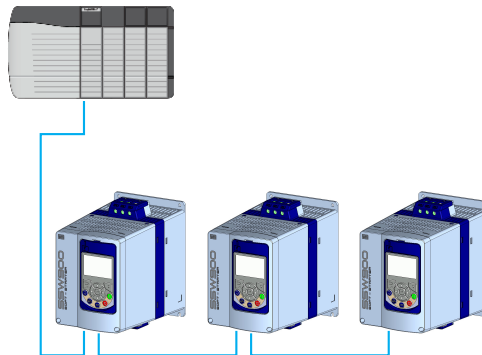
Figure 3.2: Daisy chain topology
