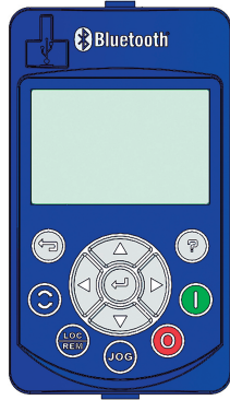
Figure 2: Bluetooth Graphic HMI
