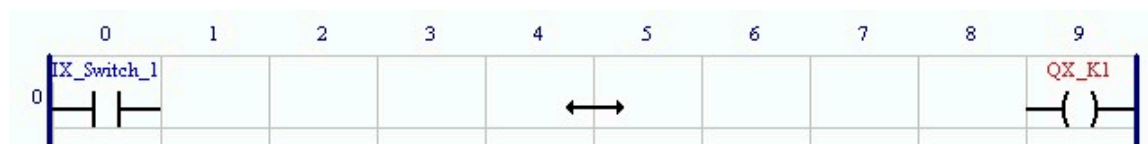
Figure – Position between NO contact and coil.
