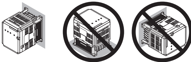
Figure 8 Correct Installation Orientation (Braking Unit)
