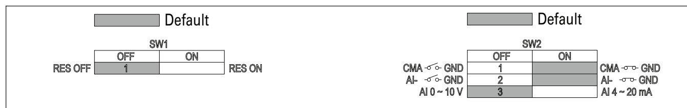
Figure 2. Termination resistor and shielding.
